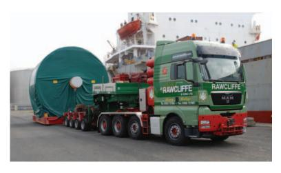
axles with drum brakes and runs on hydraulic cylinders that can be raised or lowered to distribute and level the load. "Our primary concern is the load's centre of gravity," says Rawcliffe. "If the load is heavy one end and light at the other, we need to know, so we can make sure it is distributed correctly through the axles and hydraulic cylinders onto the road.
